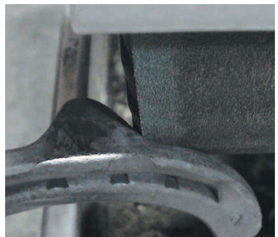
ABOVE: WORKING TOO CLOSE TO THE EDGE, WITH TOO MUCH PRESSURE MAY FORCE BELT TO SLIDE, EXPOSING RUBBER TO DAMAGE.
