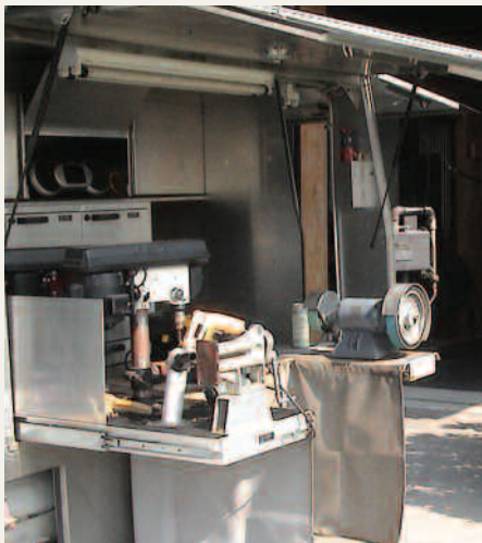
FARRIER RIG WITH GRINDER ON SLIDE-OUT
