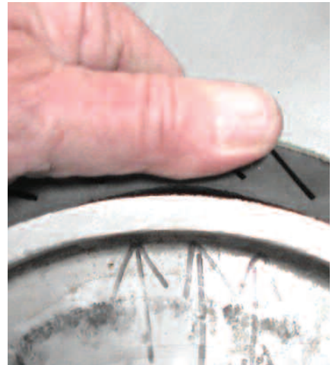
ABOVE: OPERATION OF WHEEL WITHOUT BELT CAN CAUSE DAMAGE TO RUBBER SURFACE AND MAY EVEN ALLOW SEPARATION OF RUBBER FROM METAL HUB
